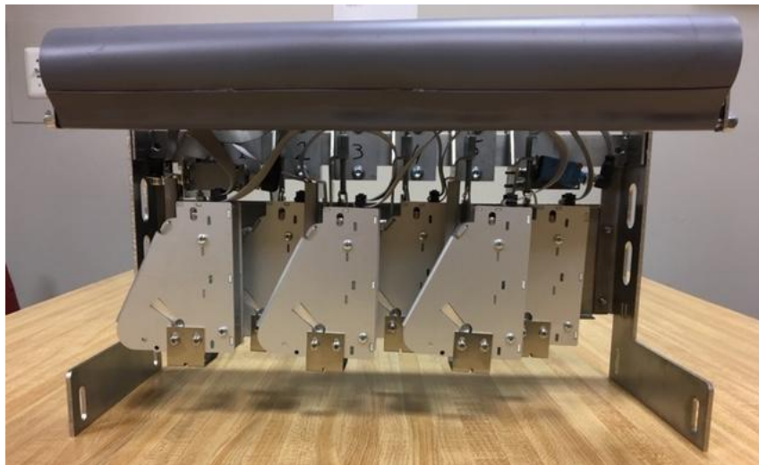
Interior view of ACCUPRINTER showing six staggered magazines for printer cartridges feeding printer heads
